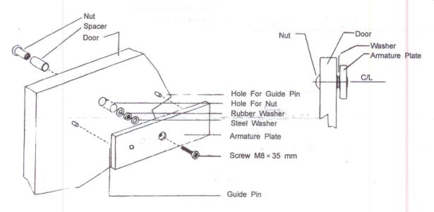
\*\*Important: Fix the armature plate not too tightly, and make the rubber washer more flexible, in order to make the armature plate automatically adjust its proper position with the magnet.
